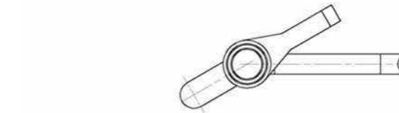
Earthing Bail enables temporary and permanent earthing of each phase conductor individually when working on insulated LV networks. It is used with all Insulated Piercing Connectors of CBS and CDRS type, except CES type. It can be used unlimited number of times. It does not contain parts which can fall off during installation. It can be delivered in a set with an Insulated Piercing Connector or separately.
